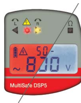
Colour change of the LCD lighting during voltage
